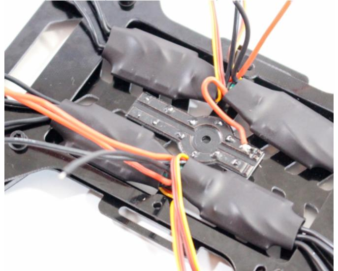
After you have the first positive lead in place, repeat the same steps to connect the negative lead from the same ESC
