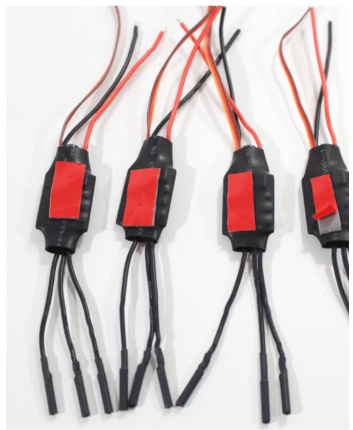
Next, position the ESCs in the subframe. Take one of the ESCs and make sure the tape is peeled back and ready for mounting. Locate the open space in the dirty frame around
