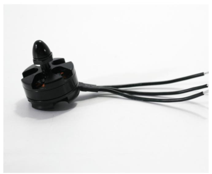
Next, use your helping hands tool to solder the male bullet connectors to the motor leads. Clamp one bullet connector into one of the alligator clips and one of the tinned motor leads in the other. Once you have everything configured, place your iron on the outside of the bullet connector, allowing it to heat up for just a few seconds before applying some solder to the inside of the connector where the wire sits.
