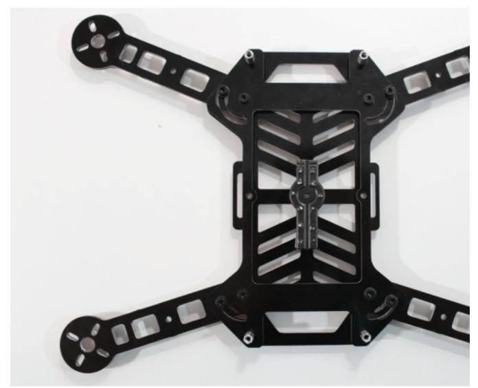
There's a 3mm hole in the middle if you'd like to add a screw for extra support. We found that the double-sided tape did a very good job and opted to not use a screw. If you do use a screw, try a small nylon screw and nut — it will save on weight and and it won't act as a conductor.
