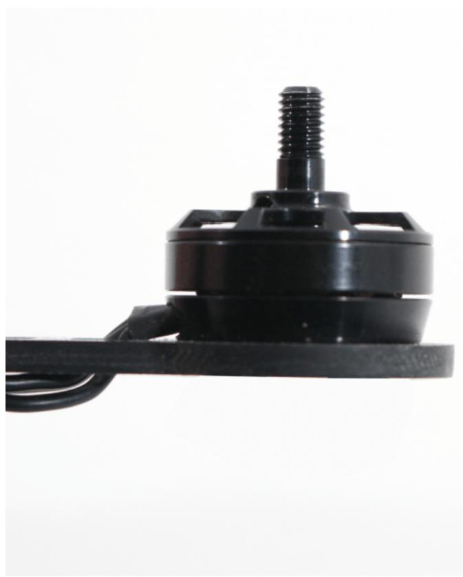
Now manually feed the first screw through the boom's motor mounting hole and into the threaded holes on the bottom of the motor. Once the first one is done, feed the opposite screw in, and keep going until you have all 4 in place.
