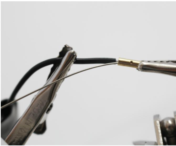
After all the connectors are soldered, cut 1" or more heatshrink to insulate each. The heat-shrink should go just to the tip of the connector while still extending over the wire on the other end, allowing the male connector to make a solid connection.
