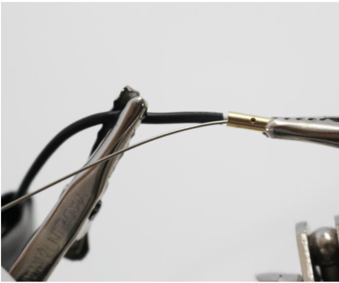
Once the solder has cooled, remove the motor lead and bullet from the helping hands and solder the other 2 motor leads and bullet connectors the same way.
