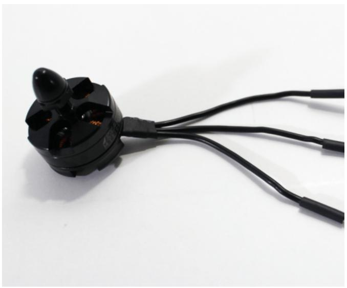
Once you have the heat-shrink in position, apply heat with your gun to shrink it. Apply this process to all 3 leads and you should end up with something that looks like the photo below.
